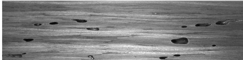
[Air inclusions in a pre-preg laminate]
