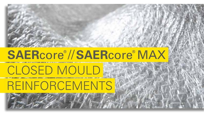
Ideal when resin injection has to be done particularly quickly: SAERcore. This patented **SAERTEX** product consists of one or two layers of chopped strand mats (CSM) and an intelligent flow media. Our multiaxial technology is integrated in our product SAERcore MAX, which reinforces the fabric complex while keeping same cavity thickness.
