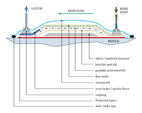
Fig. 2: Layer structure of an infusion component
