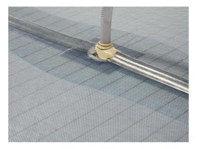
Fig. 1: Resin impregnation during the vacuum infusion process
