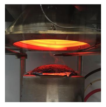
Fig. 5: Cone calorimeter test according to fire protection standard ISO 5660-1
