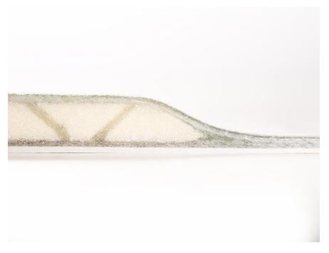
Fig. 3: Cross-section of a LEO component with a sandwich core
