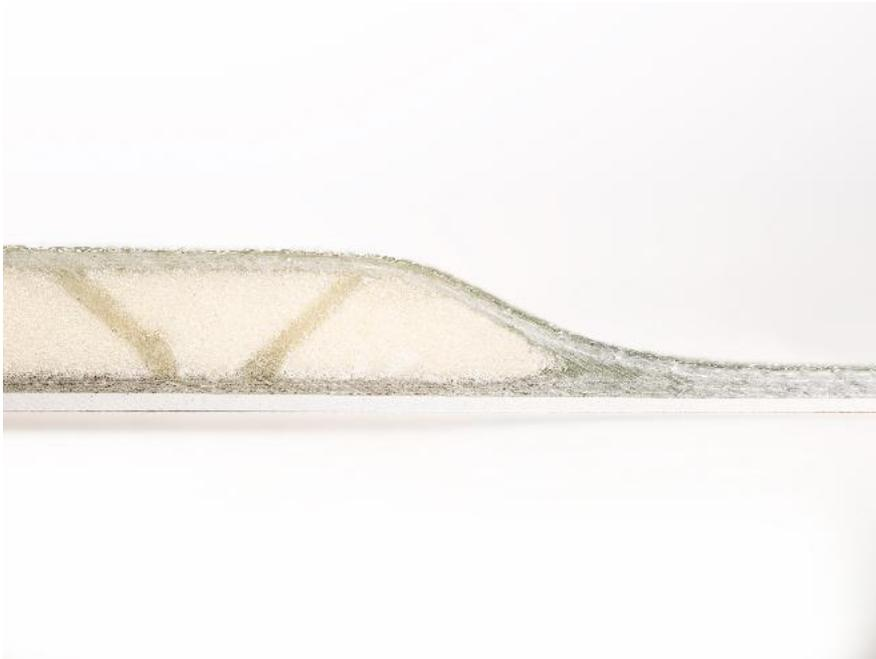
Fig. 3: Cross-section of a LEO component with a sandwich core
