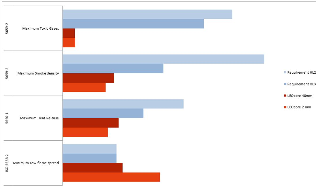
Fig. 4: Flammability results for a sandwich component with different thicknesses
