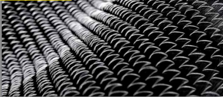
Innovative and tailor-made: **SAERTEX®** composite reinforcements made of glass, carbon and aramid fibers, also known as Non-Crimp Fabrics (NCFs). Depending on the **fiber type, surface weight and angle combination**, various mechanical characteristics can be achieved. **SAERTEX®** multiaxials are individually configured for our customers and optimally adapted to a range of processes. **SAERTEX®** NCFs are compatible with various resin systems such as Polyester, Vinylester, Epoxy or Polyurethan.
