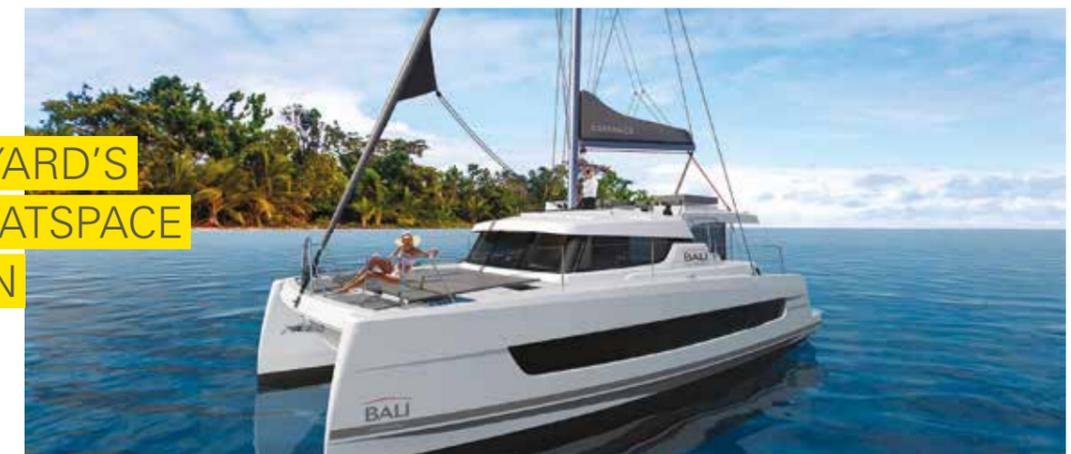
HACO Shipyard is located in Tunisia and is part of the French company **CATANA Group**, the world’s third-largest manufacturer of catamarans. **SAERTEX**® partnered with HACO to develop a new catamaran with an **entire deck produced in RTM method**. The major challenge was to produce one full catamaran every two days. **SAERTEX**® specialists had to find a way to produce an entire 12 meters x 6 meters deck in one piece using the RTM process, which would save an extensive amount of time.
