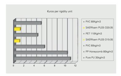
Compared products are impregnated with vinylester resin; the shear modulus is considered for rigidity.
