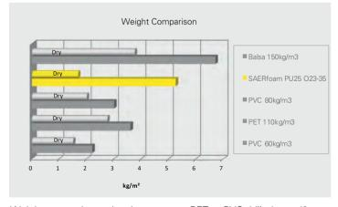
Weight comparison takes into account PET or PVC drilled core (2 mm  $\,$  / 25 mm pattern).
