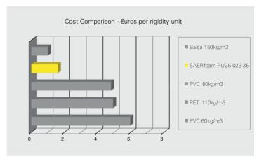
Compared products are impregnated with epoxy resin; the shear modulus is considered for rigidity.
