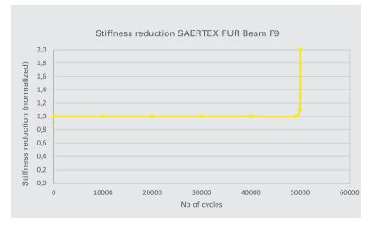
Relative change in stiffness of fatigue lifetime for low fatigue loads and high fatigue loads shows identical behavior. There is a limited linear reduction over time, but the major stiffness drop is just before failure; this specimen survived about 500,000 load cycles.
